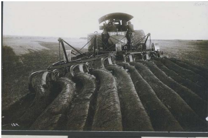
Figure 5: An image of a Reeves steam tractor turning virgin sod. Creator: Steele, F.M. (Francis Marion), 1866-1936. Date: Between 1891 and 1912. Source: kansasmemory.org .
