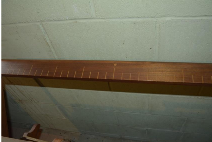
Photograph of the increments. Notice the precision and contrasting colored inlays made of maple and walnut wood. Photograph by Brandon Williams, April 8, 2017.
